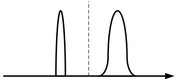
Figure 6. Low Side Injection Local Oscillator.
