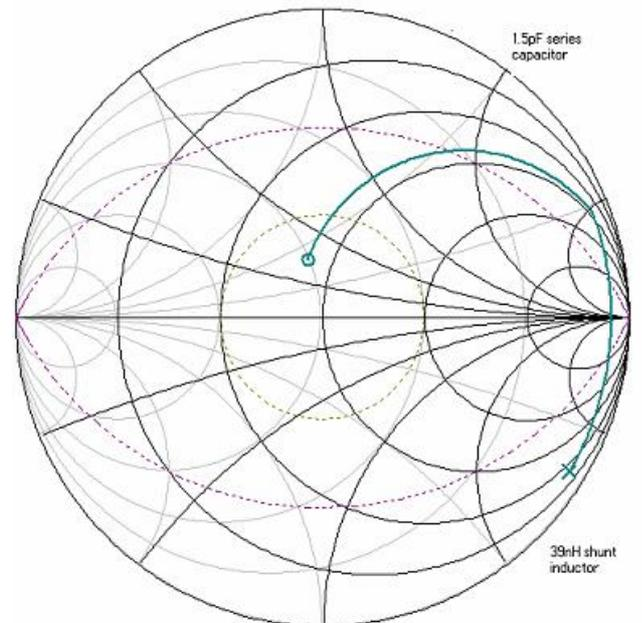
**Figure 5. Plotting the Shunt Inductor and Series Capacitor.**
