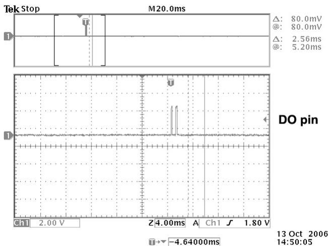
Figure 9. Data Out Pin with Squelch (SQ = 0).
